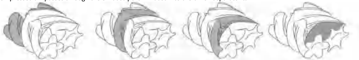
1. Inhalation process 2. Closed and conveyed 3. Compression and fuel injection stroke 4. Exhaust process
