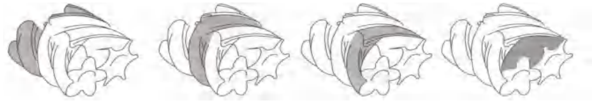
1. Inhalation process 2.Closed and conveyed 3.Compression and fuel injection stroke 4.Exhaust process
